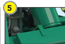
Increased cylinder rod diameter and port
