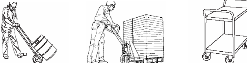
Figure 3: Keg truck, pallet truck, shelf trolley – source: Health and Safety Executive, Are you making the best use of lifting and handling aids? UK, 2005.
